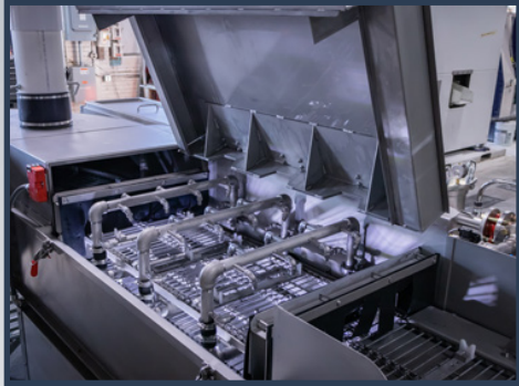
Adjustable spray nozzles give you the ability to clean high-volume parts by a continuous, flow-through wash section with 360-degree part coverage.
