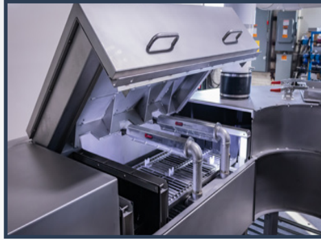
The blow-off section contains a powerful air blower to remove residual water from hard-to-reach spots on the part.
